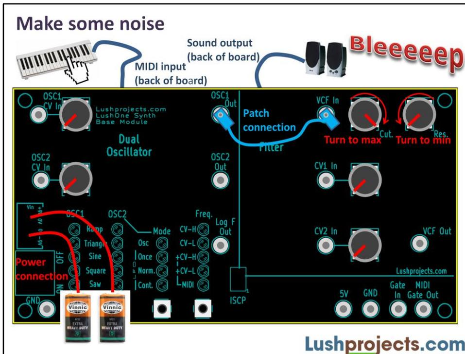
Ready to make some noise? The MIDI input and the 3.5mm output are on the back of the board. You will also of course need to connect two 9V batteries (which I won't be mentioning again!)
