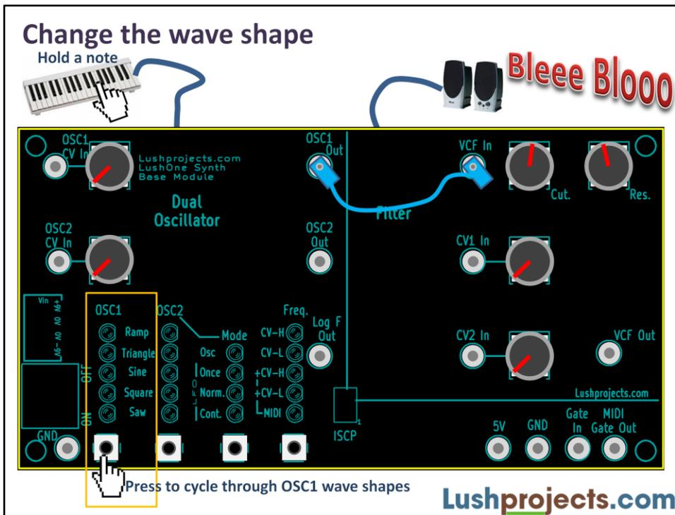
Another way to change the sound is to change the basic wave shape being generated by the oscillator. Each oscillator on the LushOne can produce a sawtooth (“saw”), square, sine, triangle or ramp wave. On OSC1 the saw and ramp will sound the same (one is the mirror image of the other and your ear can’t tell the difference) but you may want the two options for specialist effects.
