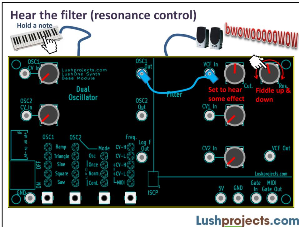
Getting the most from the filter involves using the resonance control as well as the cut-off.
