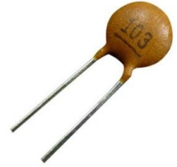
10nF Ceramic Capacitor
